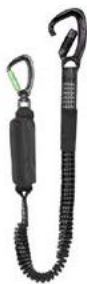
Single lanyard 2 m with energy absorber and 2 twist lock carabiners opening 20mm HAR010
