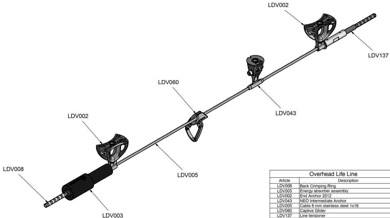
**LDV133** Glider with intermediate anchor NEO and fixing assembly. The fixing assembly enables a gap between the ceiling and the wire rope large enough to let the glider pass easily. The use of a safety block or lanyard is mandatory.
