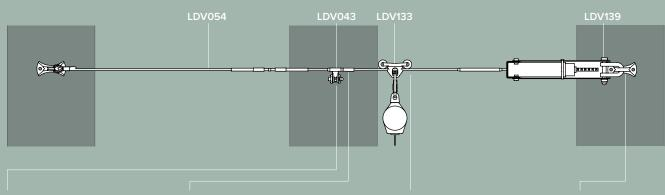
The cable guide located on a plan forming angle of 45° with the horizontal plane increases the absorbingenergy asset of the system
